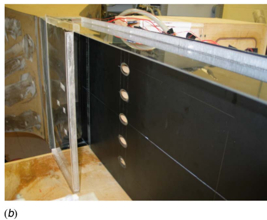
Fig. 1 Wind tunnel configuration: (a) schematic and (b) photograph of test wall with sidewalls
